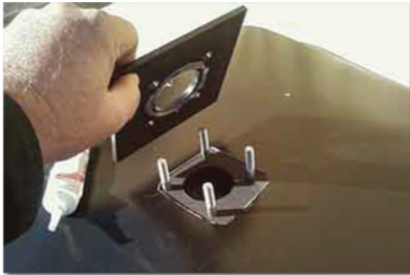
3. Install Tank Flange On Top of Bolts
