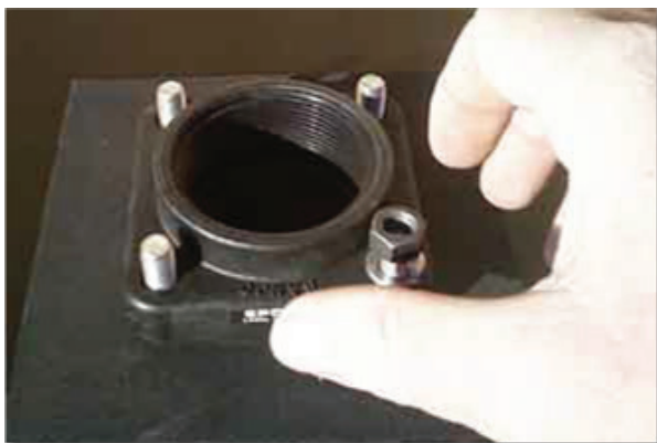
7. Tighten Nuts to Tank Flange Evenly
