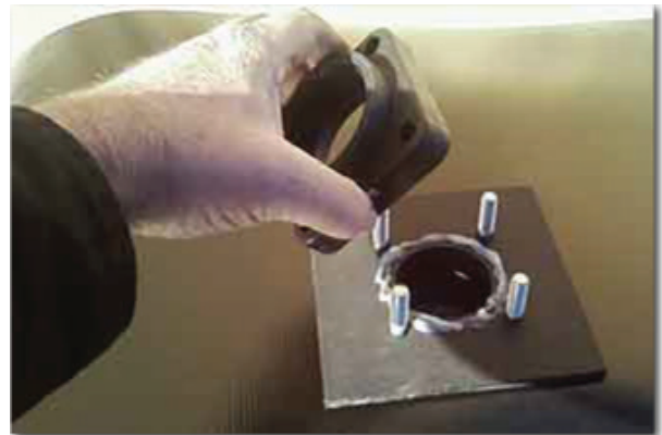
6. Install Tank Flange Fitting
